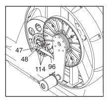
toward the rear of the elliptical exerciser until the Belt (96) is tight, and then tighten the three Button Screws.
